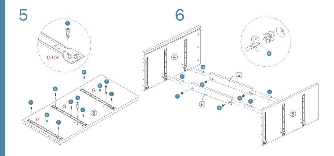
Attach 3 x right slide rails (G) to panel [5] and secure with 9 x small screws (E). Insert 2 x bolts (A) into panel [5]. Tighten with a screwdriver.
