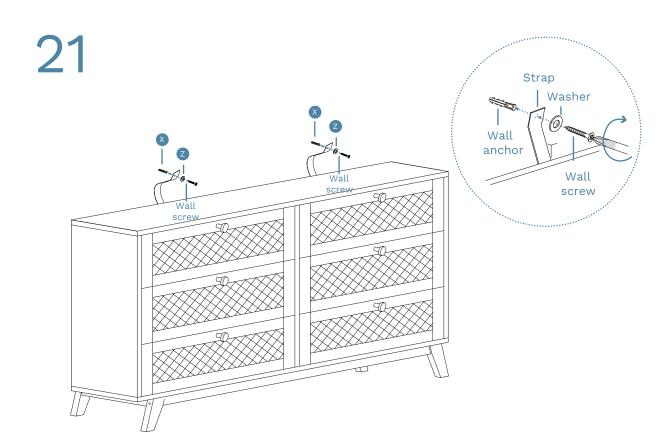
Once assembled lift furniture into place, do not drag. Use a drill to create a small hole lining up with the top of the safety stap (W). Fasten to wall using wall anchor (X), washer (Z) and screw. Ensure the unit is balaced and steady before use. You're done, enjoy!
