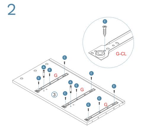
Insert 13 x bolts (A) into panel [1]. Tighten with a screwdriver.
