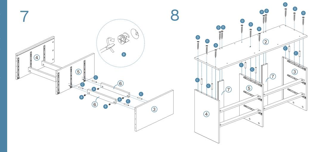
Insert 4 x dowels (C) to panels [3], [5] and [6]. Attach panels [3] and [5] to panels [6] and secure with 4 x locking nuts (B). Tighten with a screwdriver.
