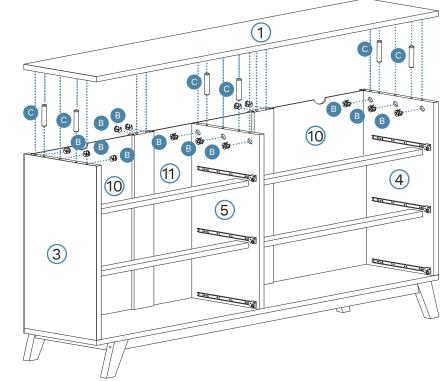
Slide panels [10] and [11] between the grooves on panels [3], [4], [5] and [7] to form the back of the unit as shown.
