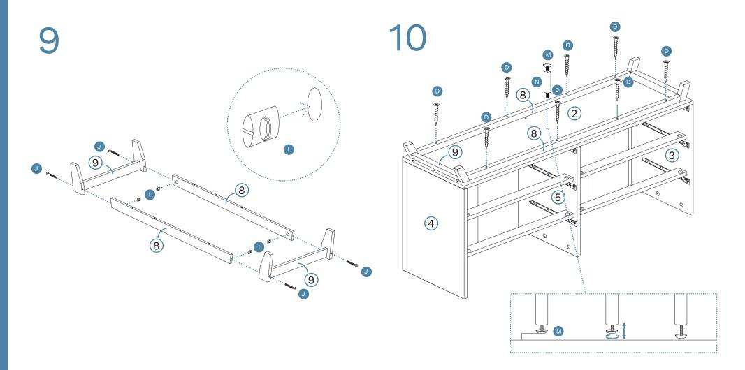
Insert 4 x nuts (I) into panels [8]. Attach panels [8] to panels [9] and secure with 4 xscrews (J). Tighten with a screwdriver.
