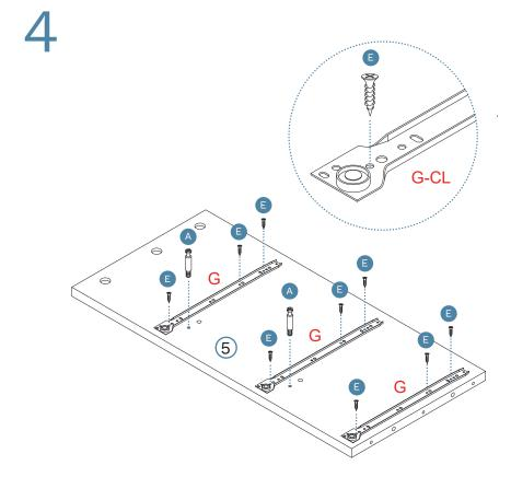
Attach 3 x right slide rails (G) to panel [4] and secure with 9 x small screws (E). Insert 2 x bolts (A) into panel [4]. Tighten with a screwdriver.
