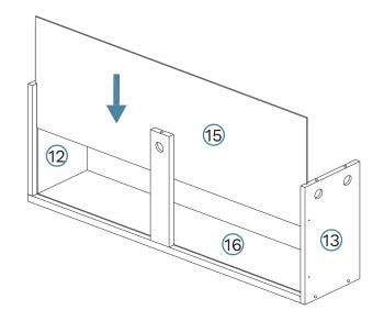
Attach panels [12], [13] and [14] to panels [16], secure with 30 x medium screws (F). Tighten with a screwdriver.
