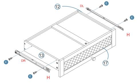
Attach 12 x slide rails (H) to panels [12] and [13], secure with 24 x small screws (E). Tighten with a screwdriver.
